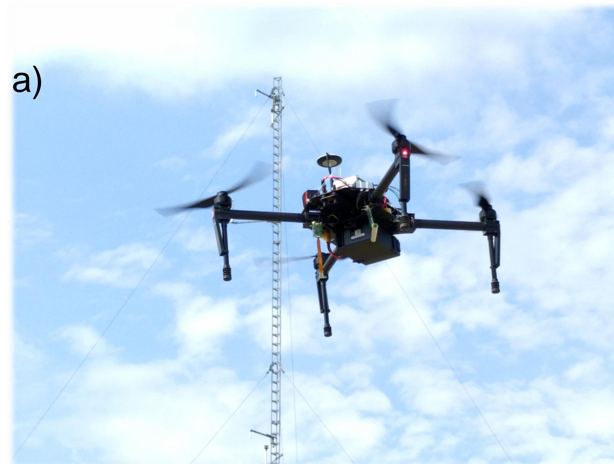
Figure 1a)-b) Drone in action. Platform used is the commercially available DJI Matrice 100 c) Close up on the SenseAir CO 2 prototype sensor HPP
