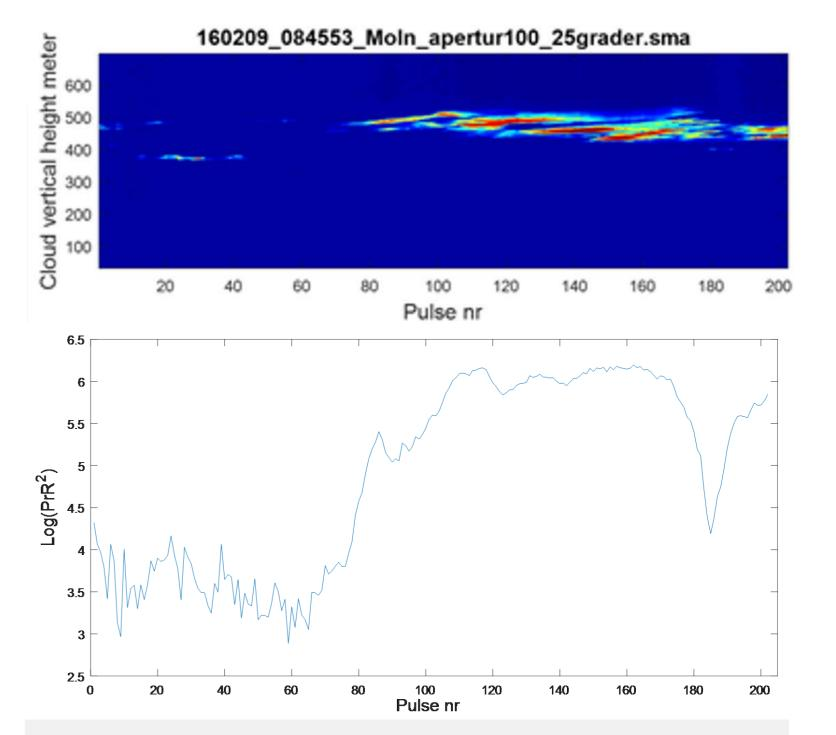
Example of cloud returns for 203 pulses. The colour coded cloud density and below the sum of  $log(P_r R^2)$  compensated signal for each waveform which correlated well with the colour intensity cloud map.
