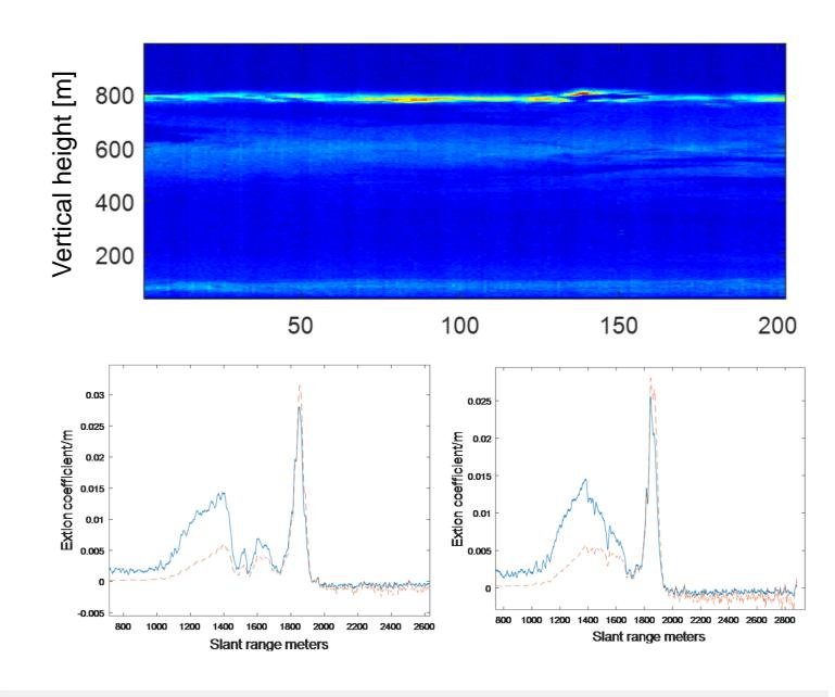
Example of a lidar data showing a thin veil below a narrow cloud layer. Example of investigations (dashed) and measured waveforms (full) to estimate the extinction variation along the cloud. The one-way integrated optical density (OD) transformed to height are 0.13, 0.15, respectively.
