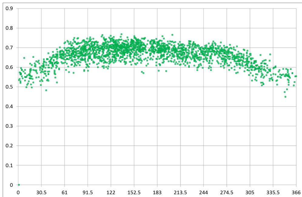
Figure 5.3 The daily relative global radiation,  $G/G_{ex}$  for “sunny days” i.e. with relative sunshine duration  $\geq 0.78$  Stockholm-KTH 1983-2018 plotted versus day-number (1-366).
