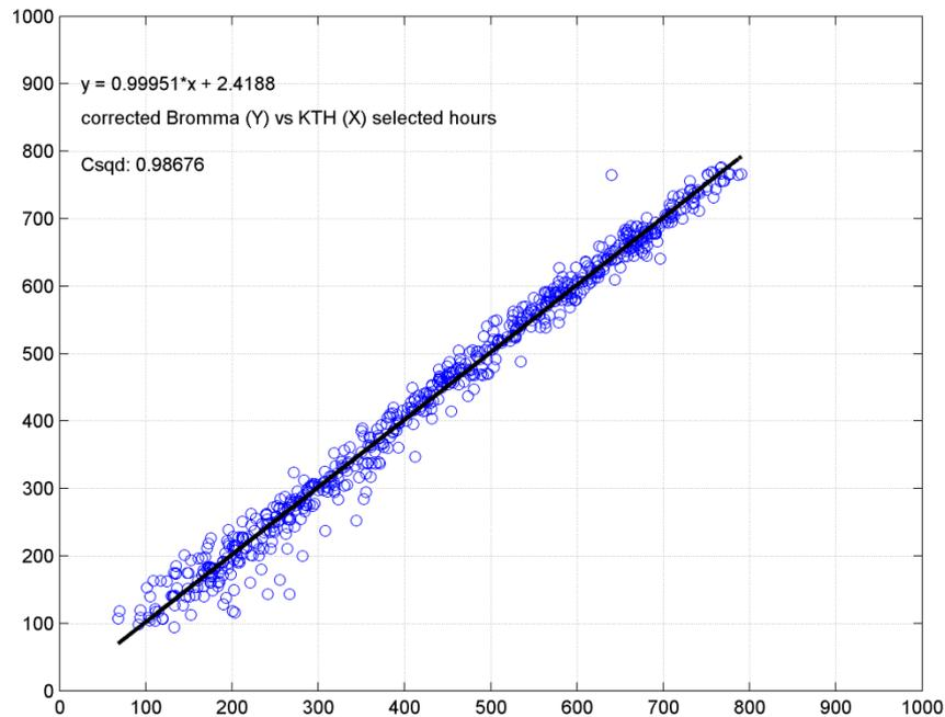
*Figure 5.5 Selected measured hourly data (sunshine duration > 59 min, global irradiation > 100 Whm-2) corrected data from Bromma plotted versus KTH. Some of the scatter remains and is due to the difference in time (true solar time was used for Bromma data and mean solar time at KTH) and to the fact that data are from two different sites. The difference in latitude is small.*
