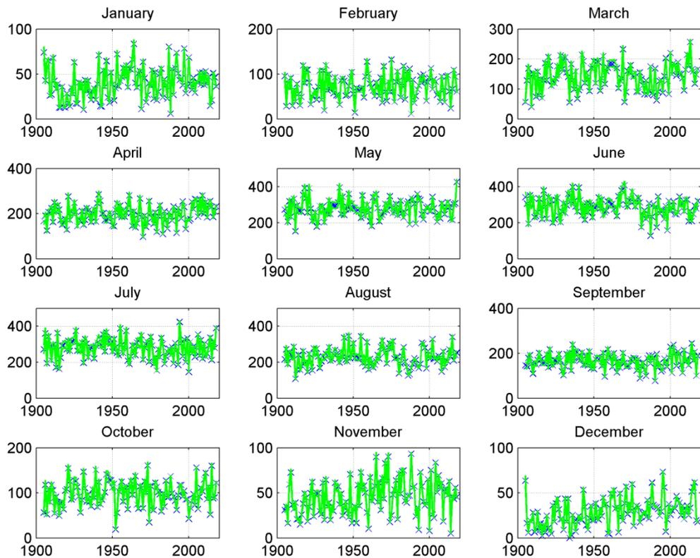
Figure A3:2 Monthly sunshine duration (hours) at Stockholm 1905-2018. Values are corrected for rime-dew effect (1905-1907, 1939-1970) and for lower sensitivity (1905-1938, 1983-1985). A rough estimate of the uncertainty ( $2\sigma$ ) is given by the range between the green lines.
