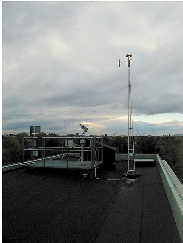
*Figure 1.1 The present location at Stockholm-KTH as it was equipped from 1983 to 2006. Since then the wind measurements have stopped and also the measurements of the direct solar radiation including sunshine duration using a pyrhelometer. The pyranometer, Kipp and Zonen CM11, is located to the left (south) on the platform.*
