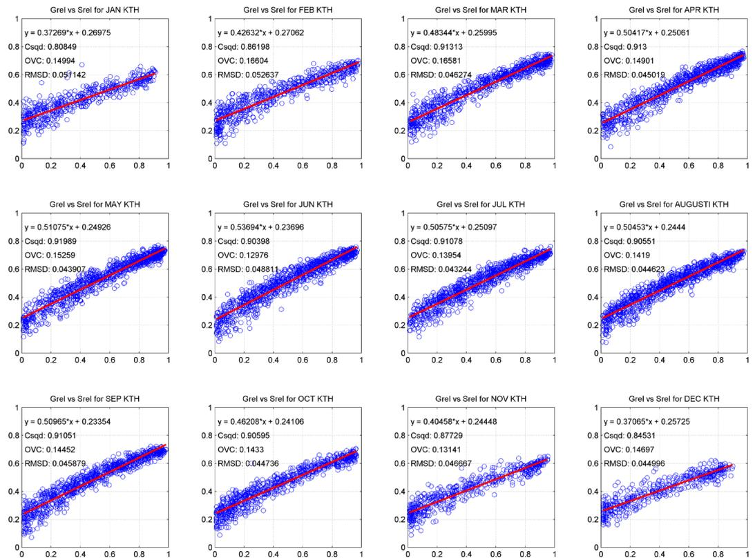
Figure 6.4 The Ångström-PreScott relation, plotted by month, for daily global radiation divided by the extraterrestrial solar radiation versus the relative sunshine duration, defined as measured hours of sunshine divided by the length of the day. In this graph all available measured daily data for the period 1983 to 2018 is plotted. Note: The measurements of the sunshine duration and the global radiation were co-located (KTH) and also co-sampled during this period.
