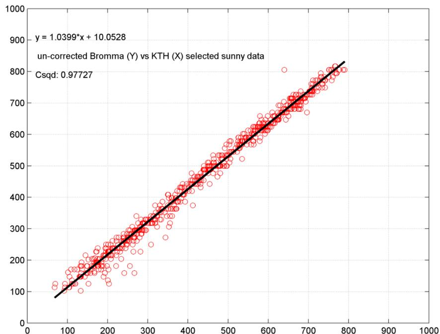
Figure 5.4 Selected measured hourly data (sunshine duration > 59 min, global irradiation > 100 Whm<sup>-2</sup>) **uncorrected** data from Bromma plotted versus KTH.
