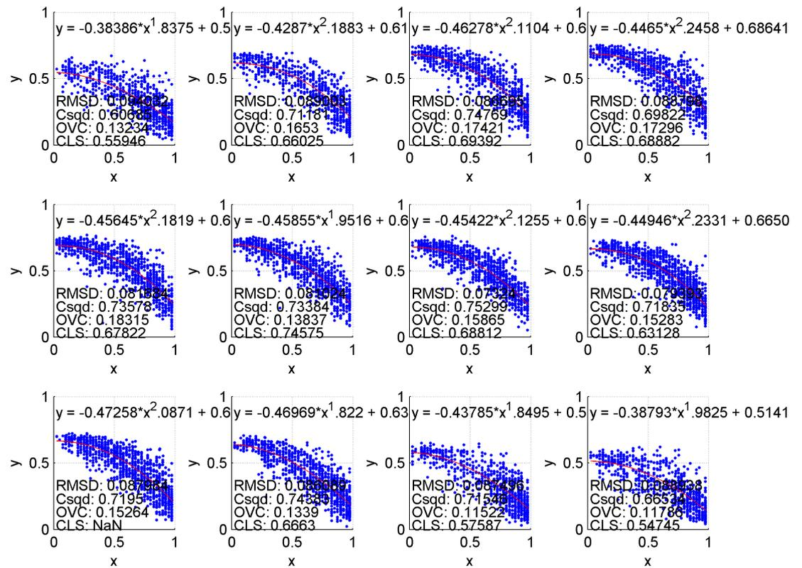
Figure 6.5 A non-linear fit (red line) of daily global radiation divided by the extraterrestrial solar radiation versus a weighted value of the cloudiness of the day for each month of the year. First row Jan, Feb, Mar and Apr etc. In this graph all available measured daily data for the period 1983 to 2018 is plotted. Note: The measurements of the global radiation and the cloud observations were not co-located; the distance is about 3 km.
