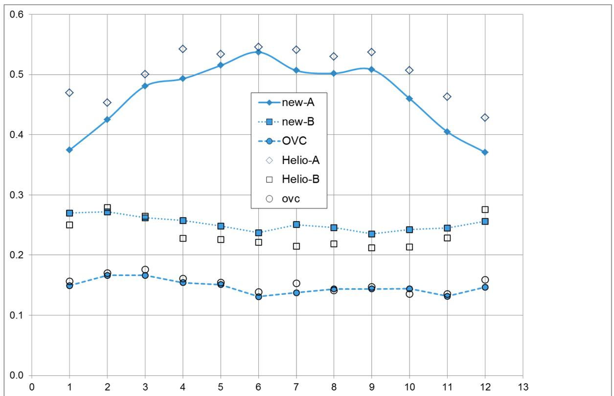
Figure 6.3 The coefficients (A and B) of the Ångström-Prescott- relation based on daily values plotted by month for two separate periods. The origin of the data can be seen in Figure 6.2 (Helio, 1952-1982) and Figure 6.4 (new, 1983-2018). The days with zero-sunshine duration are treated separately and presented as OVC which is the average of  $G/G_{ex}$  for each month (1-12).
