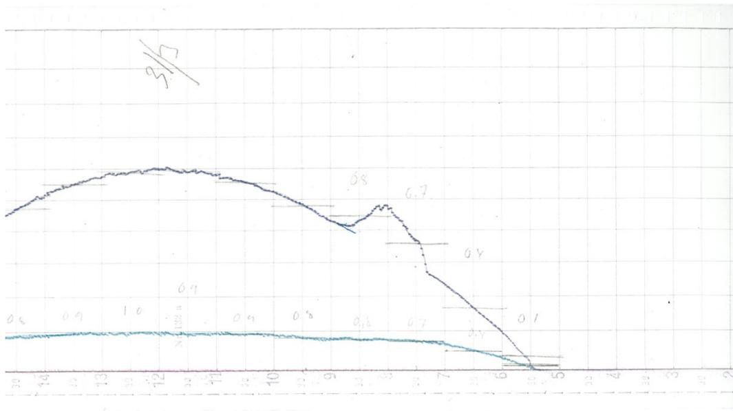
Figure 5.1 A paper roll registration from 31 March 1957. Note that time (true solar time) goes from right to left. There are three curves. The top one is the global radiation, the middle one is the diffuse solar radiation and at the bottom is a zero line from this zero-line the readings should be related, as the paper may not always be perfectly adjusted.
